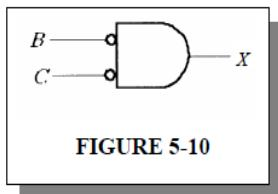
The output is dependent only on  $B$  and  $C$ . The value of  $A$  does not matter. The NOR gate behaves as a negative-AND.
