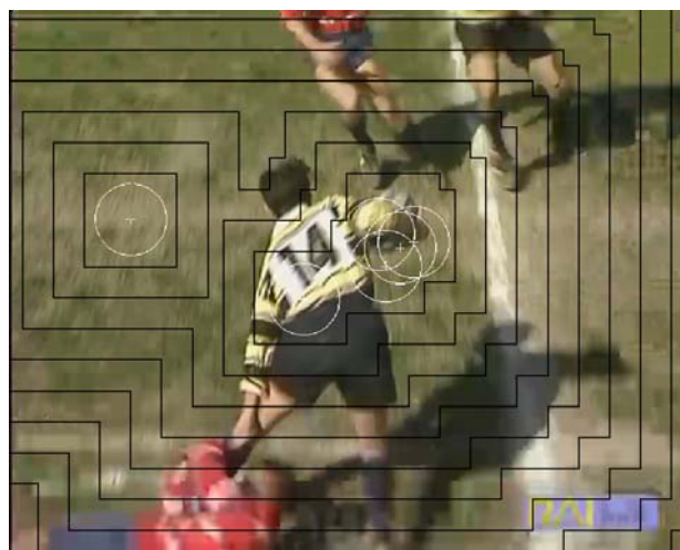
Fig 3 Use of eyegaze information to drive the encoding process. The lines show regions of constant encoding quality and the circles show regions of visual attention. The result of reducing coding quality in regions of low visual attention can be around 30% with no loss of perceived quality.
