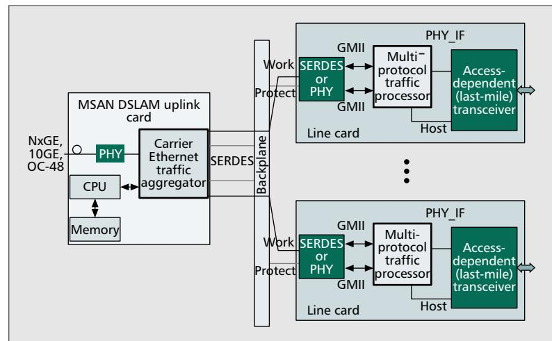
Figure 2. MSAN DSLAM architecture.
