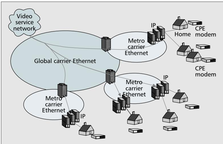
**Figure 1.** Carrier Ethernet-based IPTV network.
